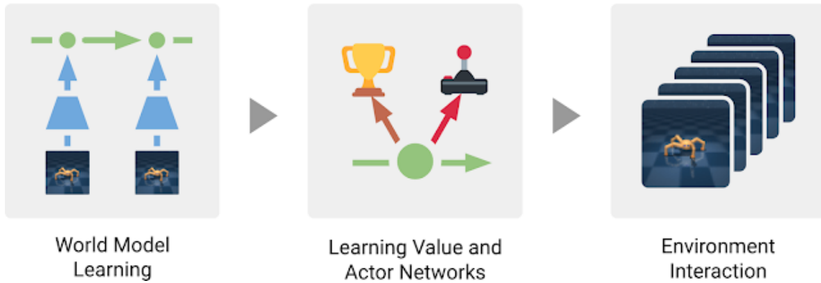
Figure 5: Dreamer’s three interleaved loops: fit the world model on replay, learn actor/value networks in imagination, collect more real data. Figure from Hafner et al. (2020).
